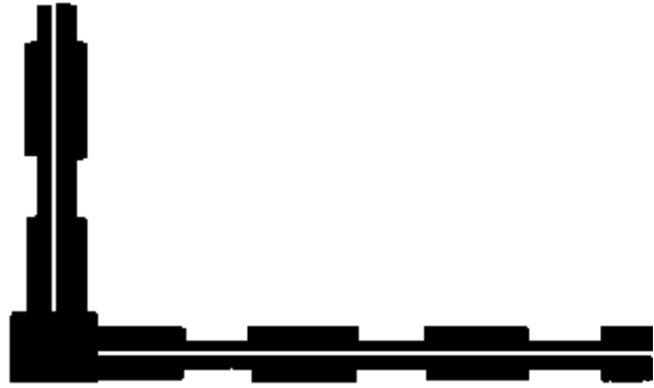
ALTERNATE BOARD Boards are in the same position on opposite sides of the stringer
